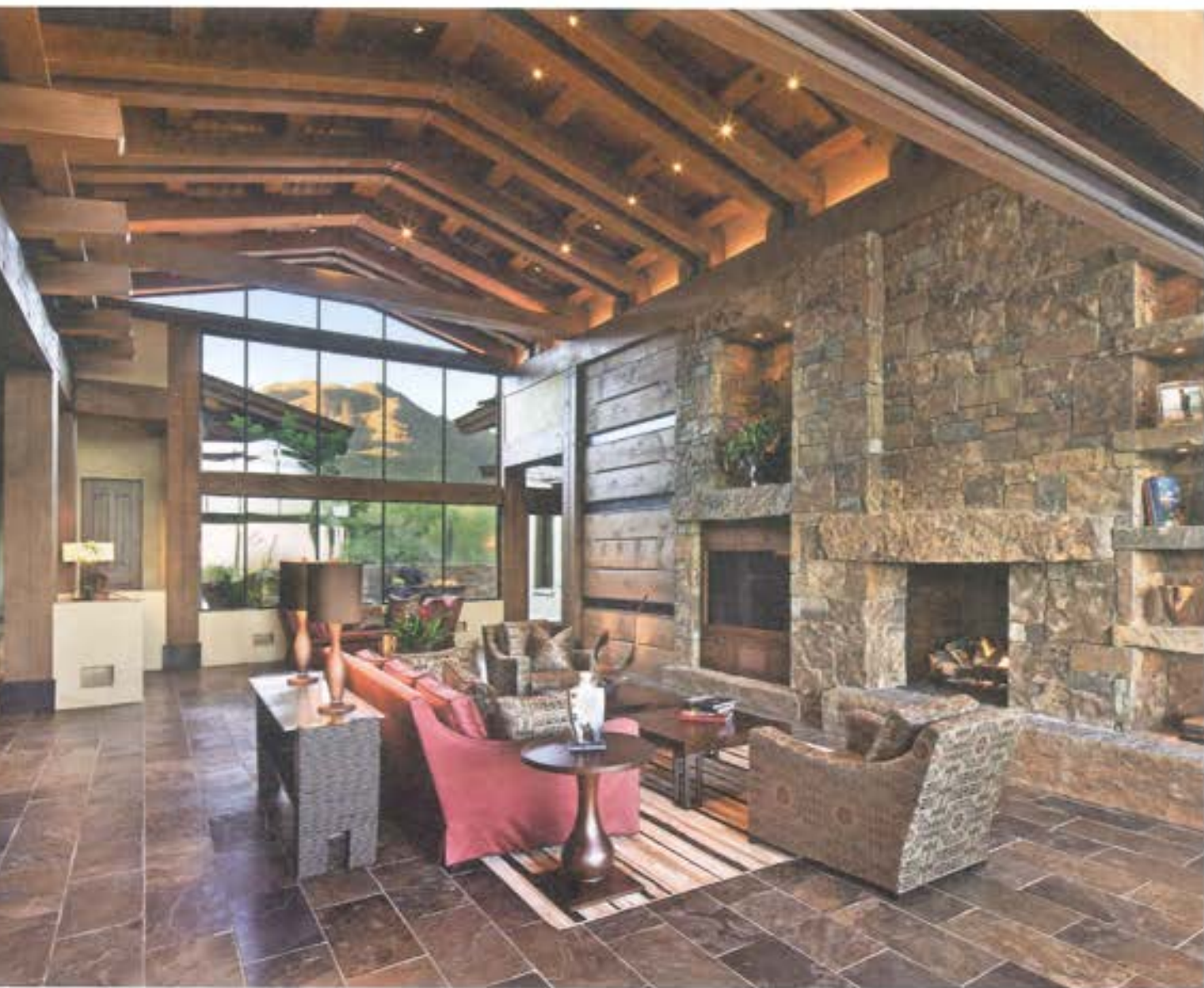
WHERE THE HEART IS The open, airy great room anchors the home, flanked by separate wings for bedroom, kitchen and dining areas. The necessary HVAC systems were carefully designed to not run through the main living spaces, but instead be concealed in the stone and timber walls.
